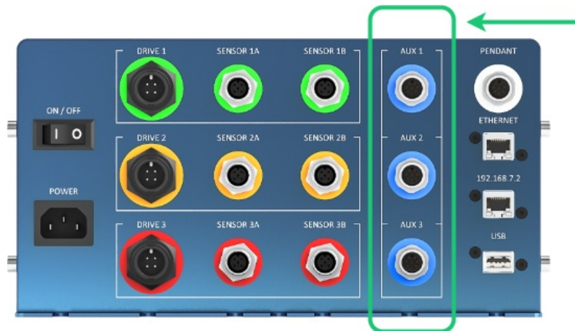
Figure 3: AUX ports on the MachineMotion1 controller
