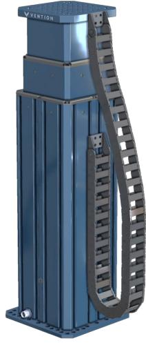
The top plate of the telescopic lift column has holes for mounting the drag chain on two sides. If you wish to install the drag chain on another side, simply remove the top plate by undoing the eight M6 fasteners and rotate the plate by 90 degrees. Reinstall the telescopic lift top plate and attach the drag chain to the side of your choice.
