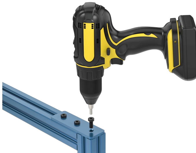
Self tapping with a drill
