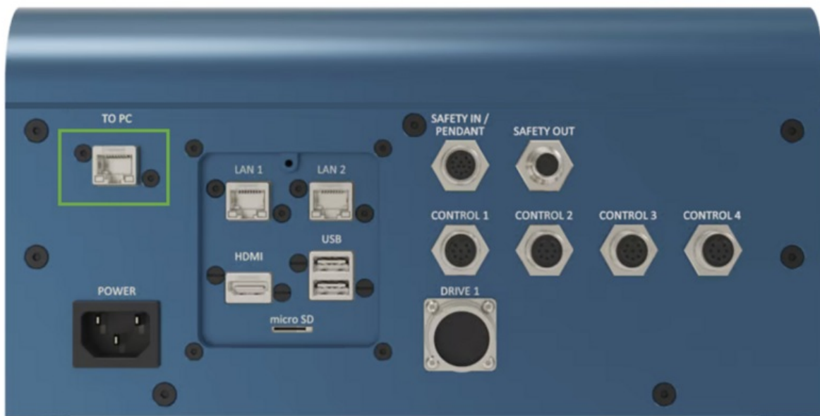
Figure 5: The "TO PC" Ethernet port on the MachineMotion controller, in the green box. MachineMotion 2 controller shown - CE-CL-010-0001.
