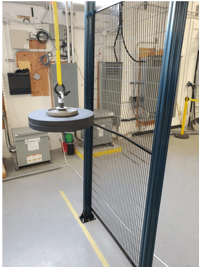
Post-impact deformation of machine guarding panel
