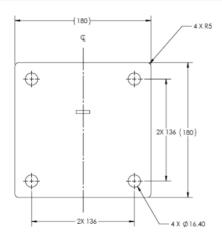
Each floor anchor has four 16.4 mm clearance holes to accommodate standard half-inch concrete anchor screws. Floor anchors also feature two layers of screws at 45 mm intervals, to maximize the number of mounting configurations.
