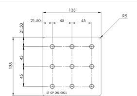
The standard Vention plate thickness is 6 mm, with the next available thickness being 11.25 mm.
