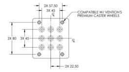
Swivel and caster wheels fit our extrusions using standard 11.25 mm thick plates. These mounting plates must have a Vention interval bolt pattern, and the bolt pattern must accommodate the swivel or caster wheel.
