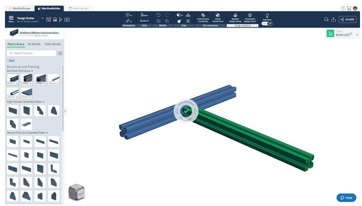
When translating a part (moving it along a single axis), the compass will show you the different number of translation options available. Use the left and right arrows to navigate through the translation options and grab the slider to move the part or group of parts.
