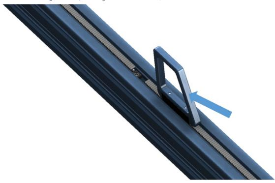
5. Once the rack segments are close, some force may be required to properly engage the segments. If necessary, adjust the set screw in step 3 so that the fit between the two segments is snug. We recomend using a soft blow hammer on the angled side of the installation tool and tapping the segment until the faces are butted together:
