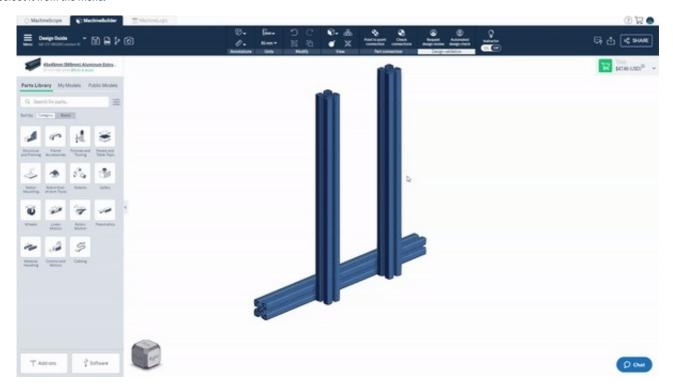
Note that the first part inserted into the 3D workspace is by default "fixed" and cannot be manipulated without removing the fixed connection. In order a float a part, the user may left-click on a part to make the "Navigation Compass" appear and then select the float icon, alternatively the user may right click and select the same action from the menu.
