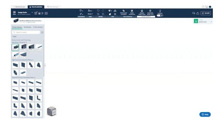
Part connection in Vention works with "automatic connections." Automatic connection options are proposed to the user a newly selected part is brought close to a previously inserted part. To confirm a proposed connection, a left mouse click is required.
