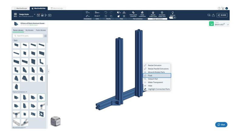
Note that at all times, a single part, or a group of connected parts, can be moved around in the 3D workspace by left-clicking and dragging them along.
