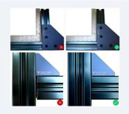
Screws are securely tightened.
