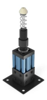
Ideally, the supporting structure should be simple, rigid, and firmly attached to the floor, as in the above example. If floor anchoring is not possible, ensure the structure can handle at least the 10 kN reaction force of the shock, with a minimum safety factor of 4.
