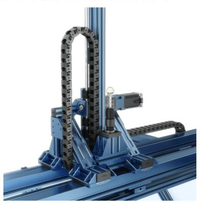
The above structure has been analysed and verified to be suitable for loads over 40 kN while the four bearings are each rated for 5 kN. This is an acceptable mounting configuration as the structure has a safety factor of over 4 and the combined bearings have a safety factor of 2. To ensure that your shock absorber mounting is appropriate, please contact Vention's application engineering team.
