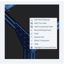
7. Part connections All parts connected. In the Navigation compass, select Float if your assembly is fixed. Move your design via drag-and-drop to identify non-connected parts.
