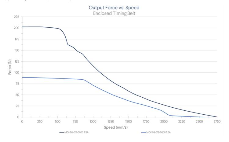
The above graph shows the output force of the enclosed axis through the range of operational speeds. Note that due to the frictional losses in the actuator, we do not recommend use of our smallest motor (MO-SM-013-0000) without a gearbox.
