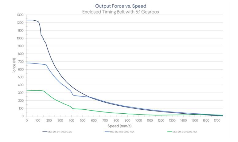
The above graph shows the driving force of the enclosed axis through the range of operational speeds when equipped with a 5:1 planetary reduction gearbox, MO-PT-001-0001. As with the earlier figure, the three different curves represent the actuator's performance with a gearbox and the three types of NEMA 34 motors offered by Vention: MO-SM-011-0000, MO-SM-012-0000, and MO-SM-013-0000, driven by MachineMotion 2.
