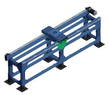
In the example above, the frame connectors and assembly plates for which all fasteners must be tightened are identified in green (one gusset and two plates).
