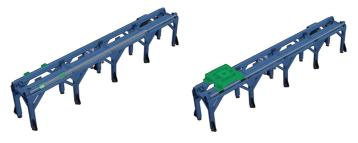
4. Move the gantry to one end of the axis and take note of any gaps or movement of the floating side. Use20mm Profile Rail Shims to fill gaps in the rails and 7/8" Slotted Shims for gaps between the frame connectors to position the floating side in a stress free position. Tighten frame connectors at the location of the gantry to lock the position of the floating side in the correct location.
