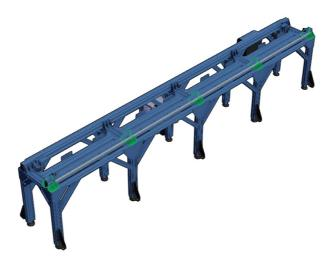
In the example above, the frame connectors on the floating side are identified in green. All fasteners in these frame connectors must remain loose.
