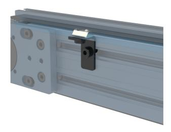
This bracket mounts to the side of the timing belt conveyor (long side) and supports the 22.5mm light-duty extrusion (short side). It is sized in accordance with the pallet and guides to ensure appropriate spacing and clearance.
