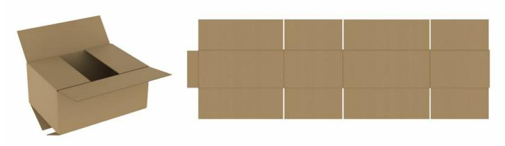
Half Slotted Container (HSC): HSC boxes are supported but box height (dimension D below) have to be between 185mm and 300mm. HSC boxes are same as a RSC but without one set of flaps.
