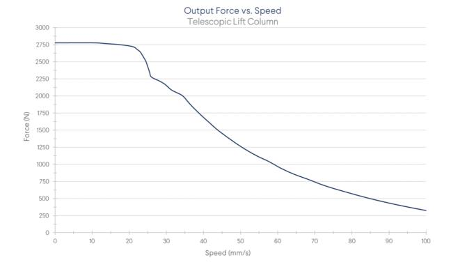
For some examples of more typical applications the following graph shows how the column can be expected to behave depending on different robots and use cases.
