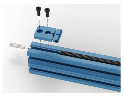
• Slide in the subsequent rack segments until all segments have been installed. This can be done by hand or by using the rack installation toolHW-TL-004-0001, and a soft blow hammer if there is any resistance.
