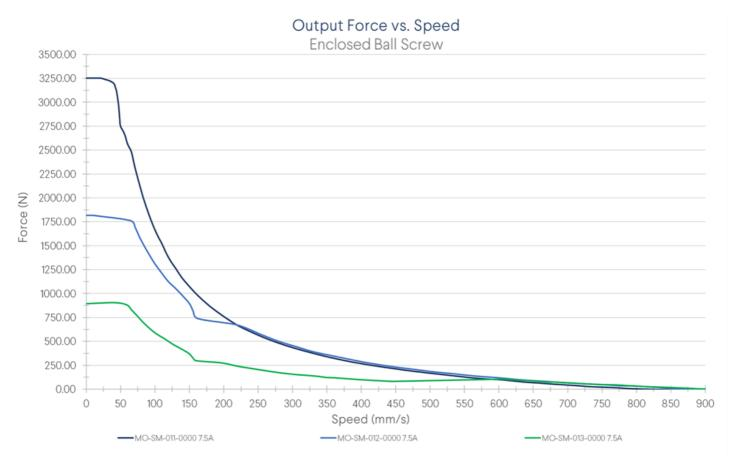
Note: During MachineMotion's boot up sequence, the holding force is momentarily 65% of its rated value. Please keep in mind when using in vertical and/or angled applications.
