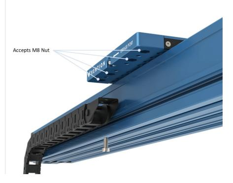
vii) Mount parts to the gantry using the threaded holes, counterbored holes or by installing nuts in the counterbored holes. The included M8 nuts easily transform the counterbored holes into threaded holes for maximum flexibility.
