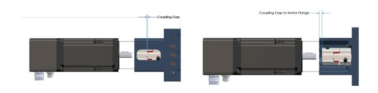
iii) After verifying the above, tighten the 4 M6 bolts that hold the motor onto the actuator, followed by the two clamping fasteners in each coupling half.
