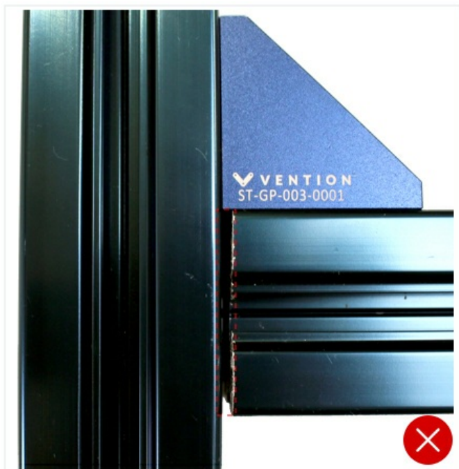
Left: Avoid creating crooked joints. Right: Check with a framing square to attain the correct perpendicular joint.
