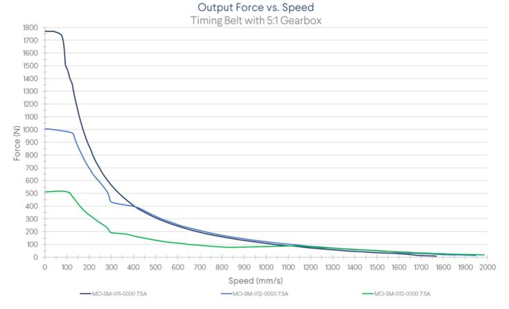
Observing the figure above, the force is much higher when using the gearbox, however it decreases much faster as the linear velocity increases. This makes the combination ideal for slower moving applications with higher forces.
