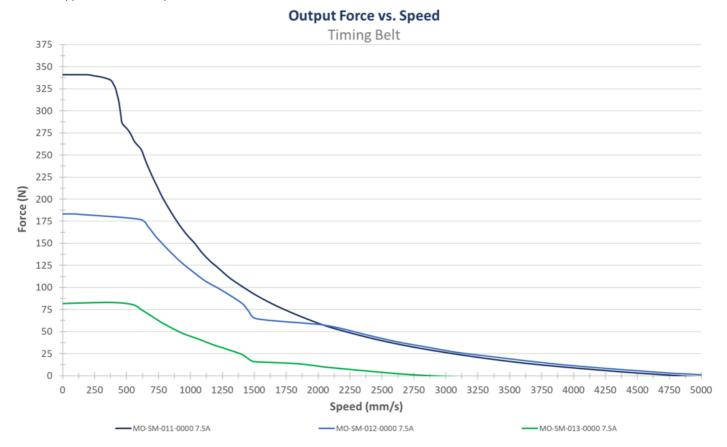
Observing the figure above, the force slowly decreases as the linear velocity increases, making the timing belt actuator ideal for lower force applications that require higher movement speeds. If more force is required and travel speed is not as critical, consider adding a gearbox to the powertrain. See the below figure for expected performance with a gearbox.
